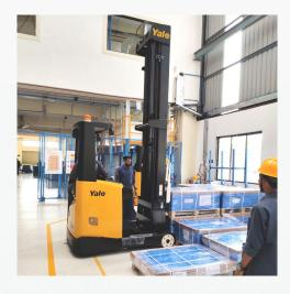
Yale® has a vast array of equipment to suit a variety of application requirements and working conditions. On carefully evaluating the requirements, our team suggested that the Yale® Reach Truck Model MR16 with 10.5m lift height will be the most appropriate equipment.
